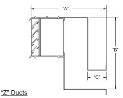
Fastened securely to vent 24 GA. galvanized steel standard. Use when space to be vented is below grade. Provide dimensions "A", "B", and "C".
